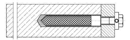
fischer anchor rod RG M with fischer resin capsule system RSB
