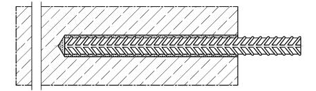
fischer rebar anchor FRA with fischer injection system FIS SB
