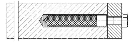
Pre-positioned installation with subsequently injected filling disk (annular gap filled with mortar)
