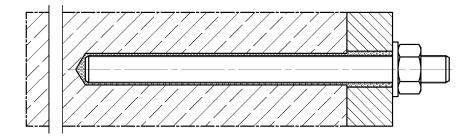
Pre-positioned or push through installation with subsequently injected filling disk (annular gap filled with mortar)
