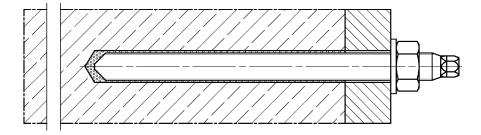
Pre-positioned installation with subsequently injected filling disk (annular gap filled with mortar)
